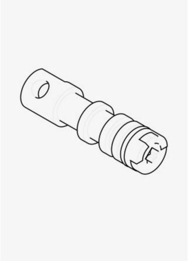
Universal Spindle Replacement Kit for Diverter and Volume Control Valve (includes 27A, 28, 29)
